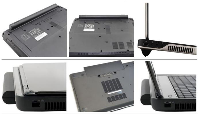
High capacity batteries (8 cell & 9 cell & 12 cell) with bigger size(shape), will protrude out the bottom or side of the laptop.
