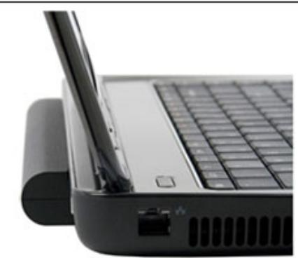
**High capacity batteries (8 cell & 9 cell & 12 cell) with bigger size(shape), will protrude out the bottom or side of the laptop.**
